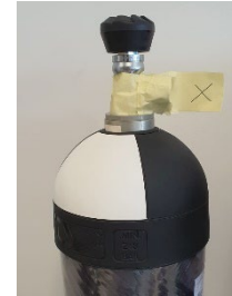
Fig.7: Cylinder with open valve and anti-tampering tape
