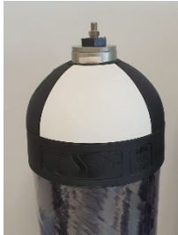
Fig.4: Cylinder with valve and internal pressure of 29 psi
