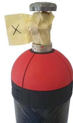
Fig.7: Cylinder with open valve and anti-tampering tape
