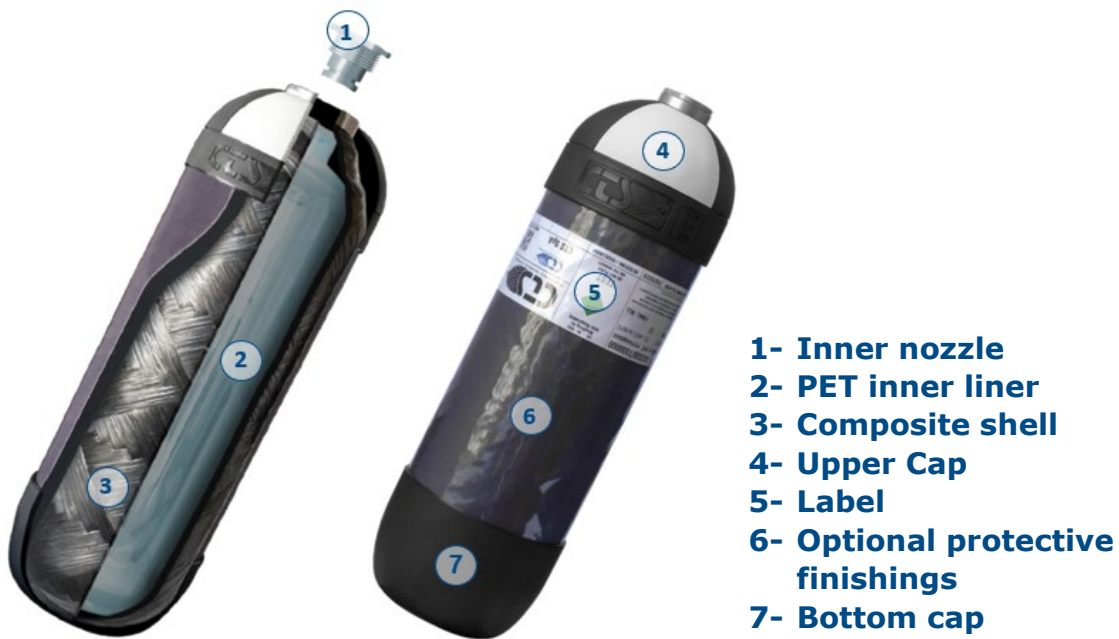
Figura 1. CTS cylinder composition diagram
