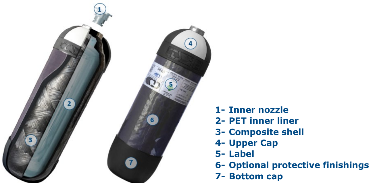
Figure 1. CTS cylinder composition diagram
