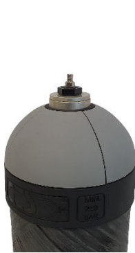
Fig.4: Cylinder without valve and internal pressure of 2 bar
