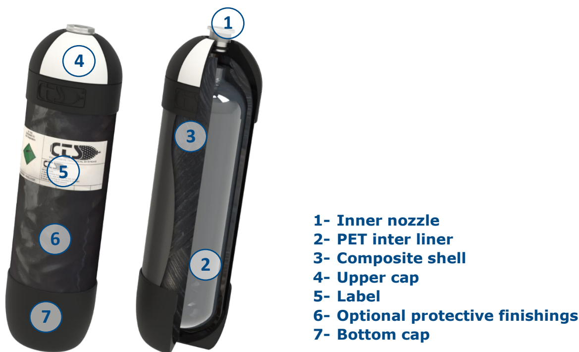
Figure 1. CTS cylinder composition diagram
