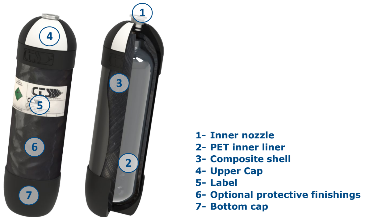
Figure 1. CTS cylinder composition diagram
