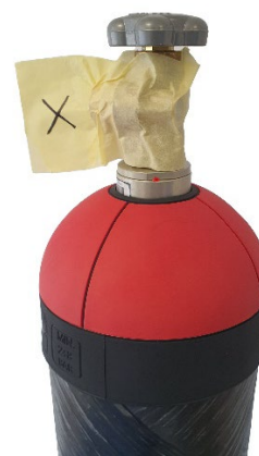
Fig.7: Cylinder with open valve and anti-tampering tape
