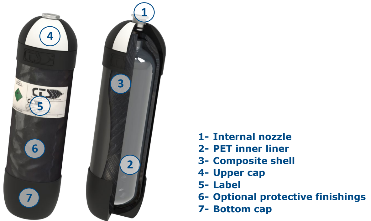
Figure 1. CTS cylinder composition diagram
