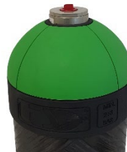
Fig.6: Cylinder with cap and without internal pressure
