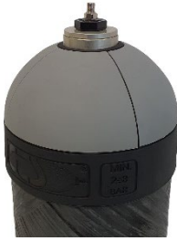
Fig.4: Cylinder without valve and internal pressure of 2 bar
