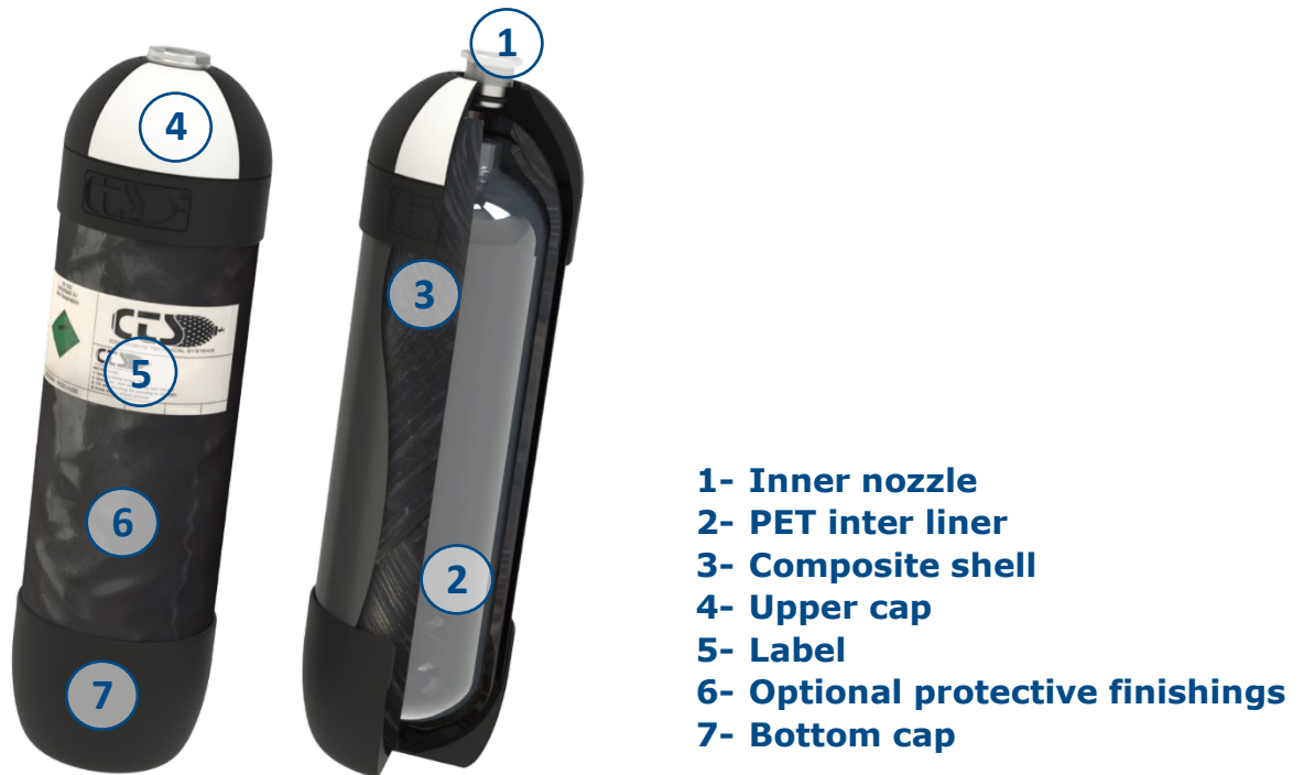
Figure 1. CTS cylinder composition diagram
